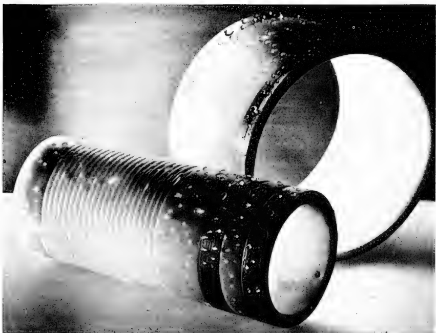
2. The water-repellent nature of the silicones. Radio coil forms made water-repellent with silicone treatment. Their surfaces are nonconducting under moisture-condensing conditions.
